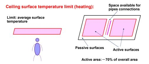
Maximum surface temperature of active area: radiant vertical asymmetry 5°C
