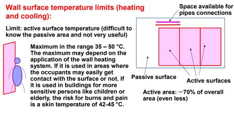
The losses to the backside must be considered.
