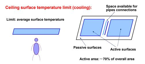
Minimum surface temperature of active area: not a question of radiant vertical asymmetry.
