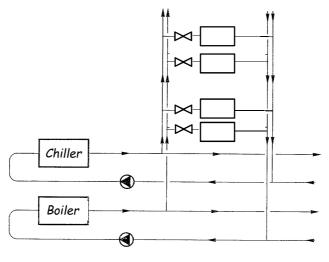
Two 3-way valves or 2 different coils
