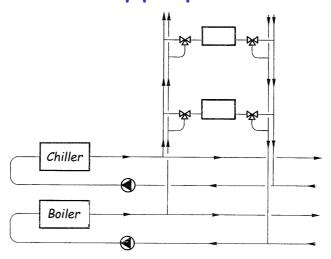
Two 3-way valves or 2 different coils
