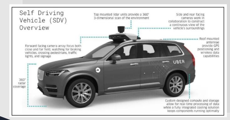
Automated Driving System designed to operate in a fully autonomous mode on premapped designated routes.
