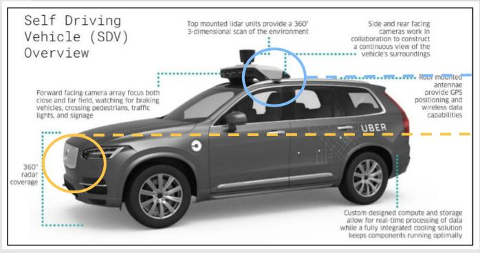
GPS and Inertia Measurement Unit for determining the vehicle's position
