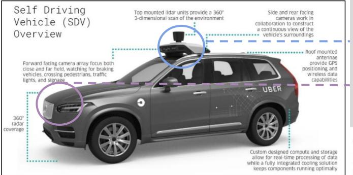
10 cameras positioned around the vehicle to provide a 360degree view of the surrounding environment.
