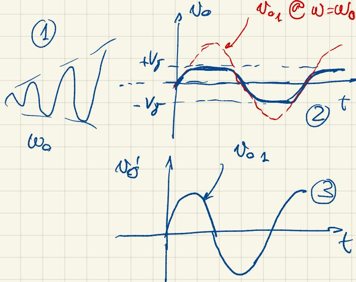
THANKS TO THE FEEDBACK OF THE RESONANT B-NETWORK  $N_O \approx N_O'$ , THE FUNDAMENTAL HARMONIC COMPONENT OF  $N_O$
