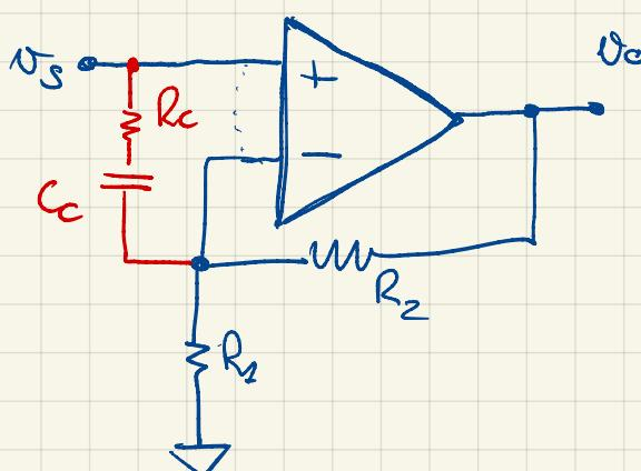
$$\text{WHEN } |T| \gg 1 \quad A_{\text{F}} = \frac{V_o}{V_s} \approx 1 + \frac{R_2}{R_c}$$
