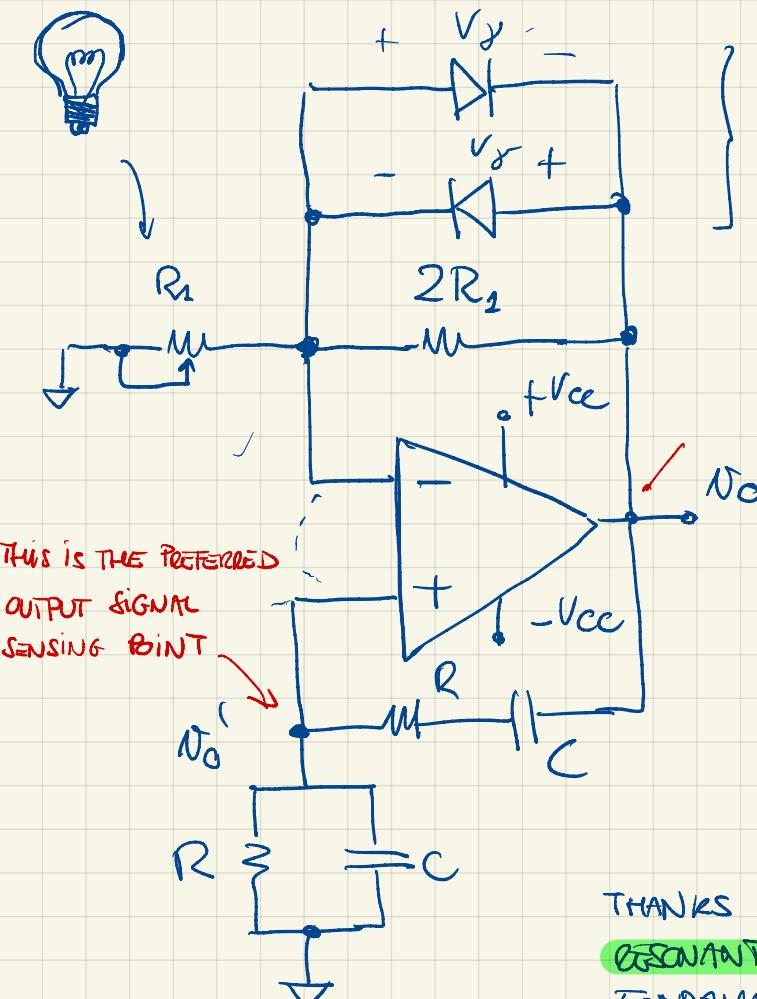
NOW LINEAR NETWORK Reduces THE CIRCUIT GAIN ANY TIME  $V_{O_0}(t)$  GETS CLOSE TO  $\pm V_D$  (THE DIODE FORWARD VOLTAGE DROP)
