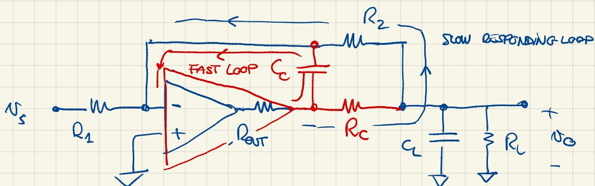
THE IDEA IS TO BY-PASS THE DECAYED FEEDBACK FEEDBACK PATH THAT STABILIZES THE AMPLIFIER TURNING IT INTO A FOLLOWER.
