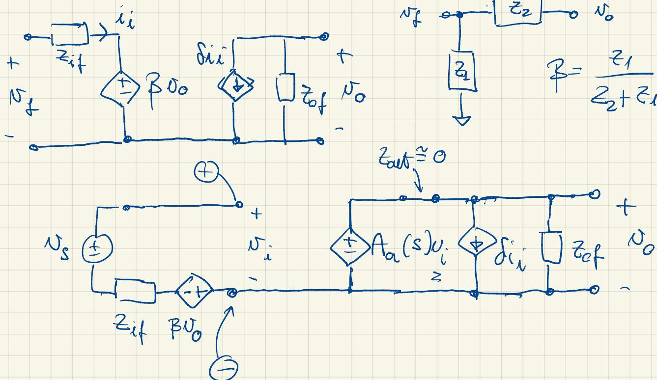
AGAIN, BECAUSE THIS AMPLIFIER HAS  $Z_{out} = 0$  AND  $Z_{in} = +\infty$  LOADING EFFECTS ARE ZERO
