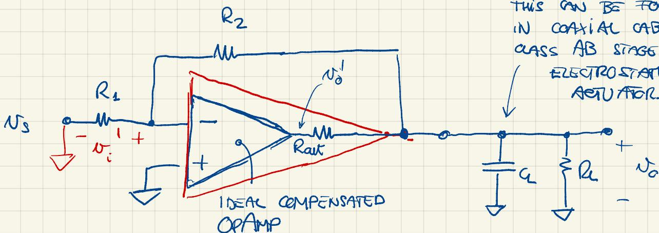
THE COMBINATION OF A CAPACITIVE LOAD AND  $R_{out} \neq 0$  IS GOING TO GENERATE STABILITY PROBLEMS.
