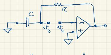
$$T = \frac{v_e}{v_t} = -\left(-\frac{A_{\alpha\beta}}{1 + \frac{s}{\omega_0}}, \frac{\frac{1}{sc}}{R_+}\right) = \frac{A_{\alpha\beta}}{1 + \frac{s}{\omega_0}}, \frac{1}{1 + sRc}$$
