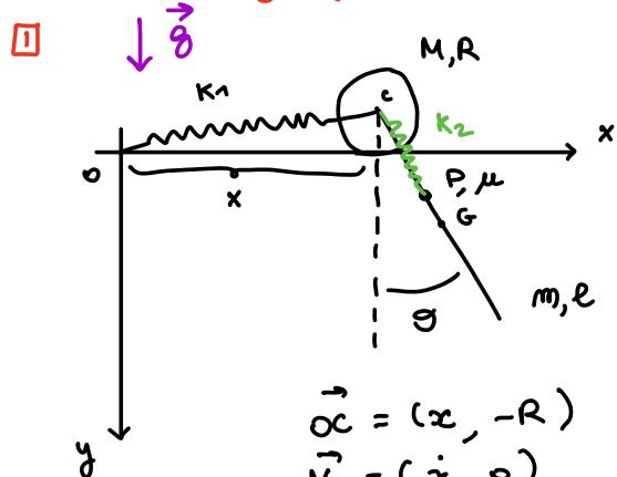
disc bar : rotates without sliding
