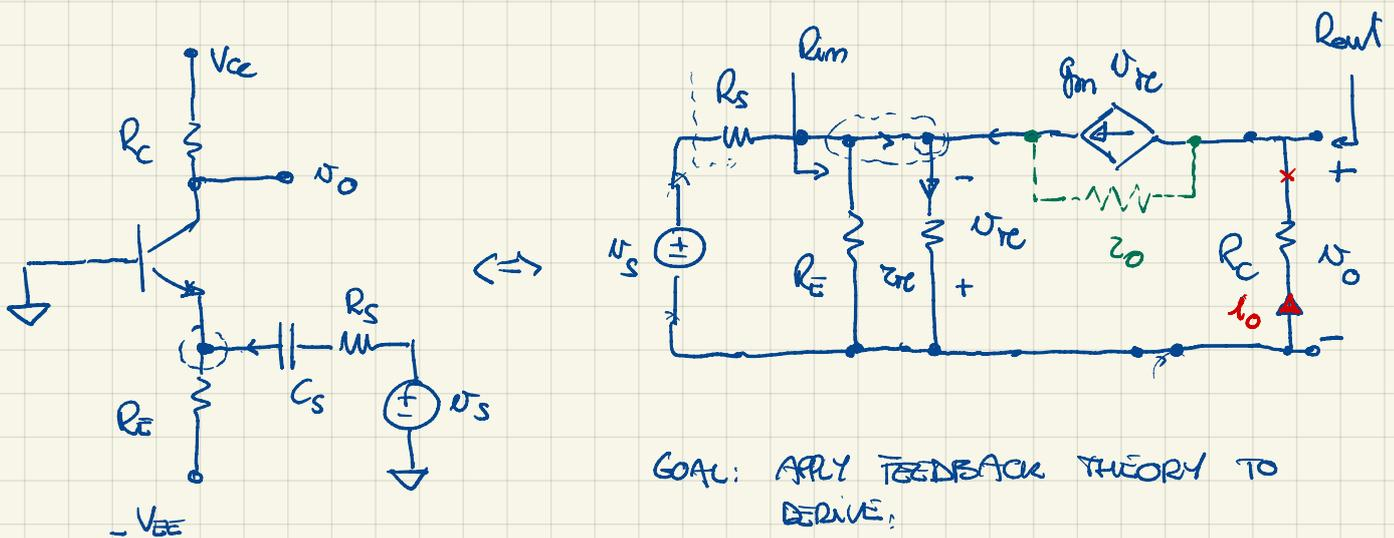
$$A_v \triangleq \frac{v_o}{v_s}, \quad R_{in}, \quad R_{out}$$
