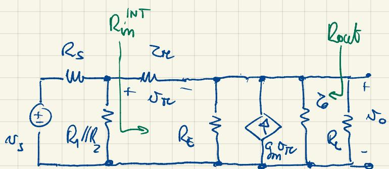
THE SMALL SIGNAL EQUIVALENT CIRCUIT CAN BE "EASILY" SOLVED:
