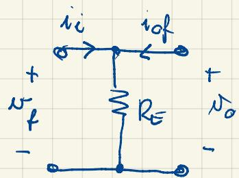
TWO TWO PORT EQUIVALENT MODEL OF THE  $\beta$ -NETWORK IS: THAT OF A VOLTAGE AMPLIFIER (SERIES-SHUNT) :
