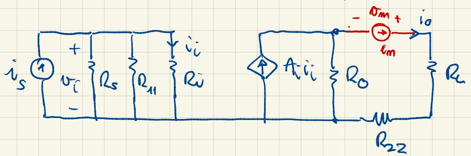
$$A_i^a = \frac{i_o}{i_s} = \underbrace{\frac{R_s || R_{11}}{R_s || R_{11} + R_i}}_{\alpha_i} \cdot A_i \cdot \frac{R_o}{R_o + R_{22} + R_L} = \alpha_i A_i \alpha_o$$
