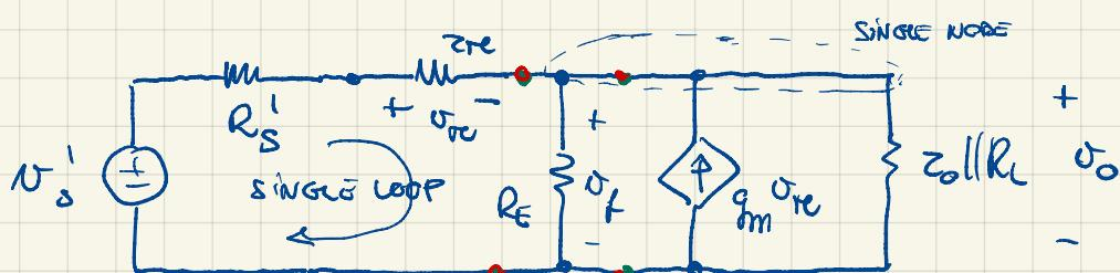
$$u_s' = \frac{R_1 \parallel R_2}{R_s + R_1 \parallel R_2} u_s$$
