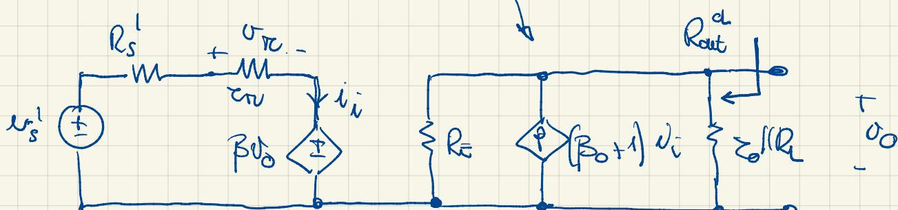
FROM THIS CIRCUIT WE CAN FIND OPEN LOOP PARAMETERS BY SETTING  $\beta = 0$
