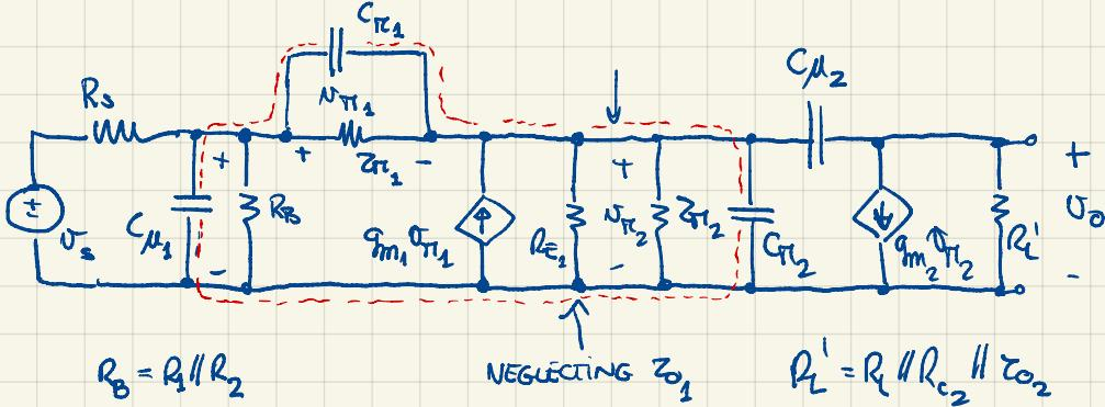
$$R_{in1} = R_{in_{CC}}^{\text{INT}} = Z_{T1} + (\beta_0 + 1) R_{E1} // \underline{(R_{in2})} \quad \text{LOADING EFFECT!}$$
