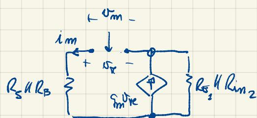
$$v_m = (R_s // R_B) i_m + R_{E_1} // R_{\text{out},2} (i_m - q_m v_m)$$
