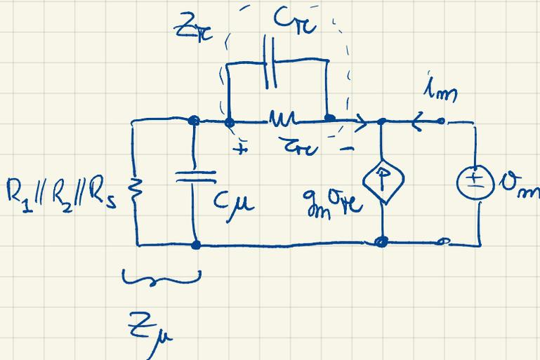
$$\begin{cases} i_{tm} = - \left( g_m v_{re} + i_{z_{re}} \right) = - v_{re} \left( g_m + \frac{1}{z_{re}} \right) \\ v_{re} = - \frac{z_{re}}{z_{re} + z_{\mu}} v_{tm} \end{cases}$$
