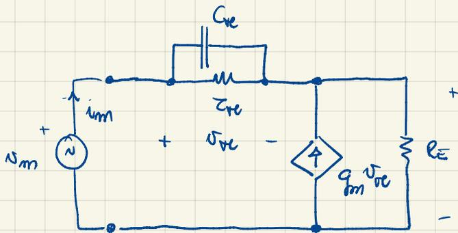
$$v_{\pi} = Z_{\pi} i_{tm}$$
