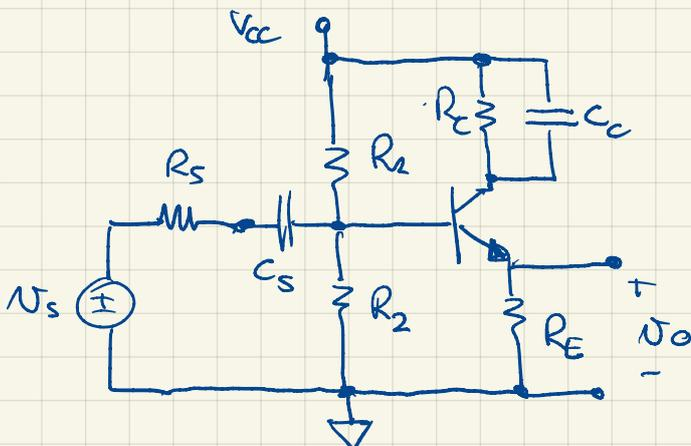
IF ALL CIRCUIT PARAMETERS ARE KNOWN, WE CAN FIND THE BIAS POINT ( $V_{CE}, I_C$ ) AND THE SMALL SIGNAL CIRCUIT PARAMETERS LIKE  $g_m, z_o, C_{\mu}$  ...
