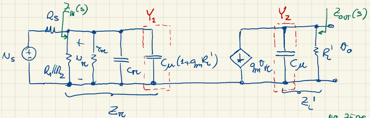
$$A_{V, HF}(s) = -\frac{Z_{re}}{R_s + Z_{re}} \cdot g_m \cdot Z_L' = -\frac{R_{re}^0}{R_s} \cdot \frac{g_m R_L' \left( \begin{smallmatrix} \text{NO ZEROS} \\ \cdot \end{smallmatrix} \right)}{(1 + s R_{in}^0 C_{in}) \cdot (1 + s C_{\mu} R_L')}$$
