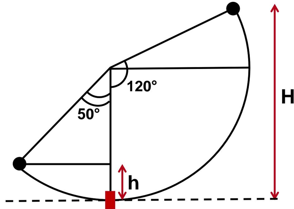
$$P = \text{peso mazza} = 5,1 \text{ kg} \cdot 9,81 \frac{\text{m}}{\text{s}^2} = 50 \text{ N}$$
