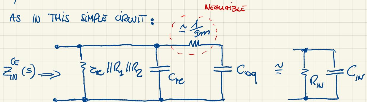
$$R_{in} = r_{re} \parallel R_1 \parallel R_2$$
